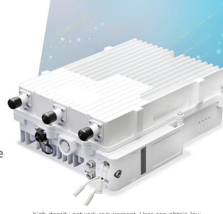
high density network requirement. User can obtain low latency and up to 400 UE connections. It is the best 5G integrated small base station in telecom industry. NX-R2028 integrates CU, DU and RU into a lightweight all-in-one machine which greatly reduces the complexity of network deployment and has comprehensive advantages such as flexibility and rapid deployment.
